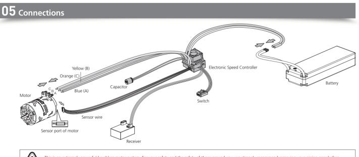
This is an extremely powerful brushless motor system. For your safety and the safety of those around you, we strongly recommend removing your pinion gear before erforming calibration and programming functions with this system, and keeping wheels in the air when you turn on the ESC.
